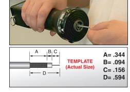
Remove the Mylar foil only from segment "B" (segment "B" only, maintain Mylar foil over segment "A").
